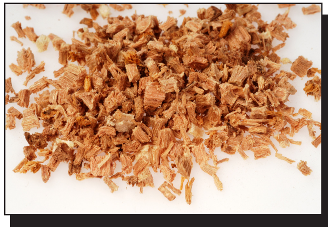
Figure 4—Wood shavings from the Tuatahi crosscut saw are short.
