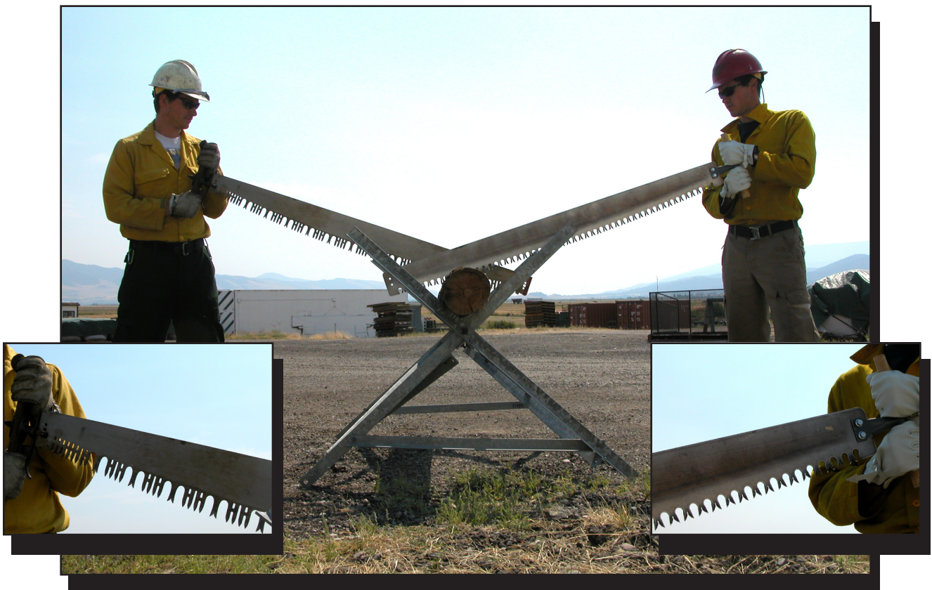
Figure 1—A vintage perforated-lance tooth, peg-and-raker crosscut saw (left) and the M tooth Tuatahi Homesteader saw (right) were field tested on forests across the country.
