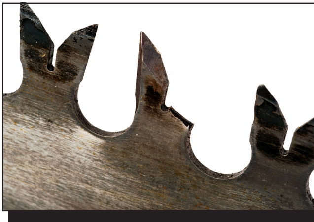
Figure 6—A tooth broke on the Tuatahi Homesteader saw when a log fell on it. The manufacturer and the U.S. supplier say this problem has not occurred before.
