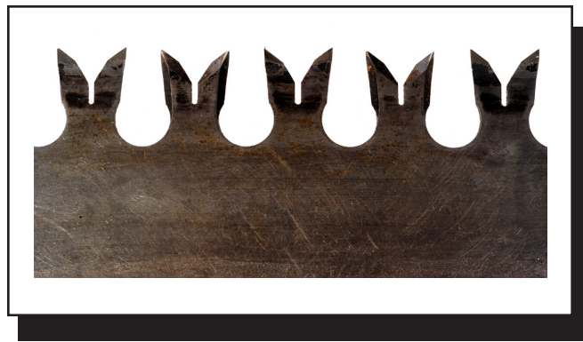
Figure 3—The M tooth pattern on a modern Tuatahi Homesteader crosscut saw.
