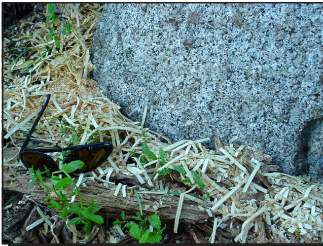
Figure 5—The shavings from a peg-and-raker crosscut saw are much longer.
